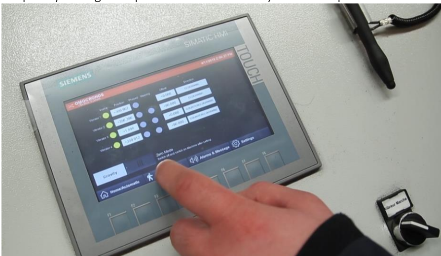
View of the OMOCRONOS vibrating table control screen
