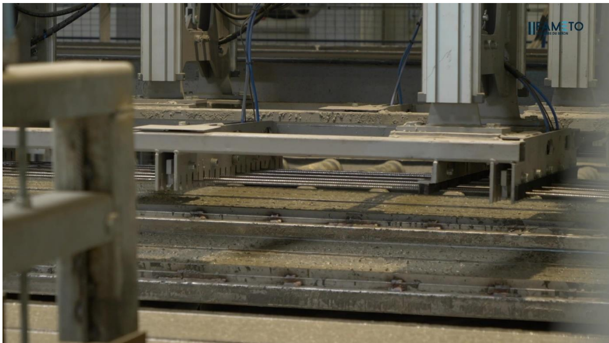
7. Automatic steel setting according to product.
