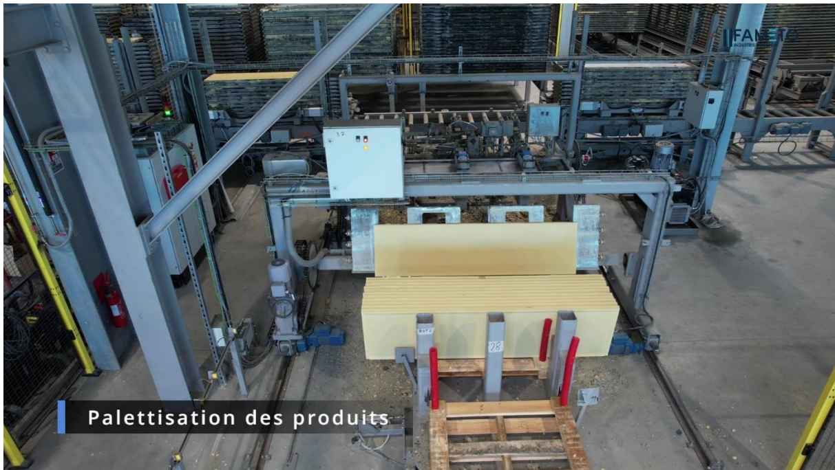
10. Automatic bridge to insert wooden pallets into the demoulding stations and manage the exit of complete pallets.
